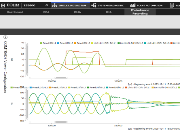
Figure 8. Comtrade Viewer for Fault Monitoring and Analysis
